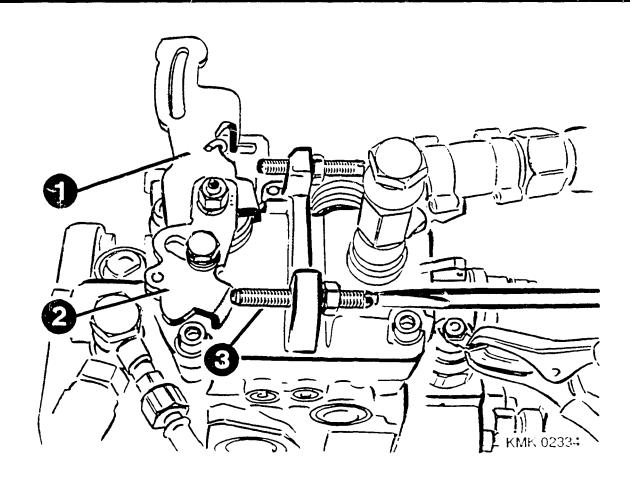
ADJUSTING CONTROL-LEVER POSITION "XK"
